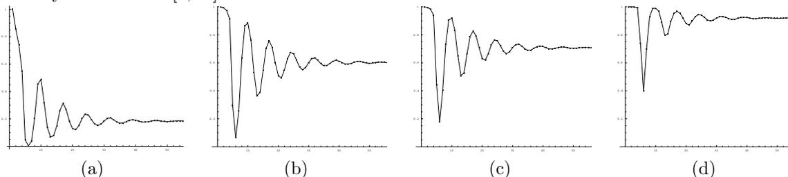
Figure 2: Availability of the (a) series system, (b) 2-out-of-3:F system, (c) consecutive-2-out-of-3:F system and (d) parallel system.
