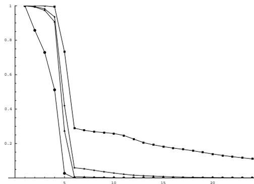
Figure 1: Reliability  $R(k)$  of the four systems. The reliability of the series system is depicted by circles, of the parallel system by boxes, of the 2-out-of-3:F system by triangles and of the consecutive-2-out-of-3:F system by stars for  $k \in [0, 50]$ .
