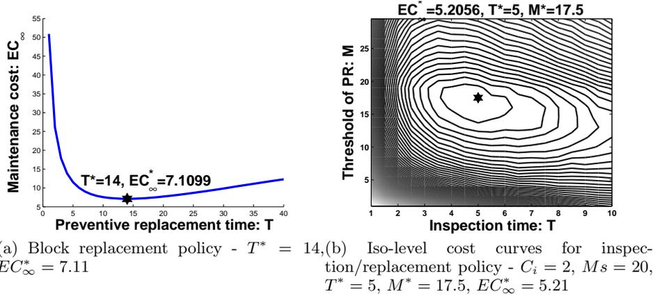
Figure 1: Optimal values of maintenance policies for  $\alpha = \beta = 0.1$ ,  $L = 30$ ,  $M_s = 20$ ,  $\lambda_1 = 0.01$ ,  $\lambda_2 = 0.1$ ,  $C_p = 50$ ,  $C_c = 100$ ,  $C_d = 25$
