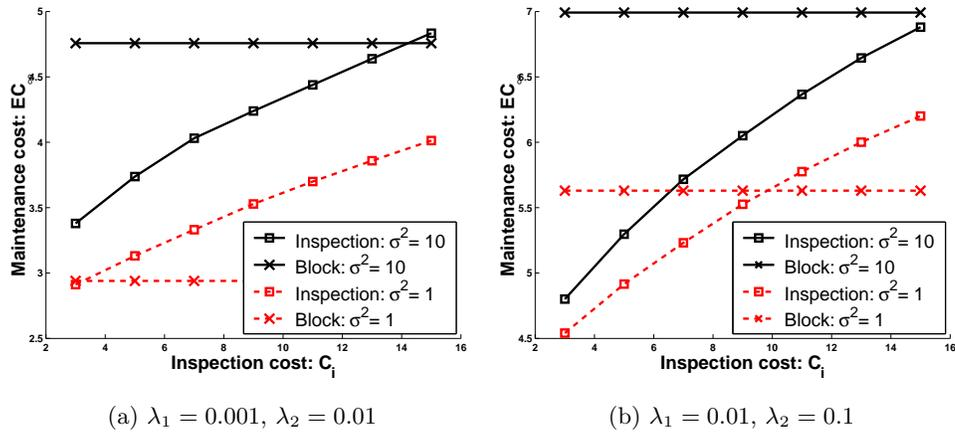
Figure 2: Comparison of the policies maintenance costs as a function of the inspection cost  $C_i$  -  $L = 30$ ,  $M_s = 20$ ,  $C_p = 50$ ,  $C_c = 100$ ,  $C_d = 25$
