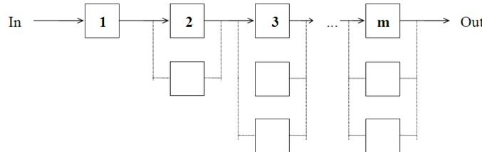
Figure 3: Series configuration of a m-stage production system
