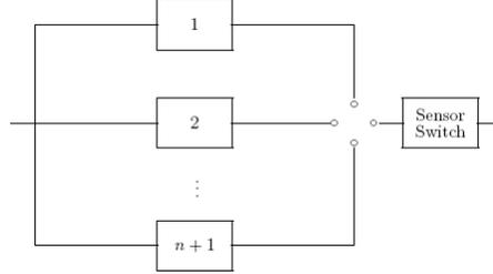
Figure 1: System configuration with n standby components, one switch and one sensor
